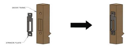
INSTALL STRIKE PLATE TO THE INSIDE OF THE DOOR FRAME WITH (2) SCREWS (NOT SUPPLIED).
